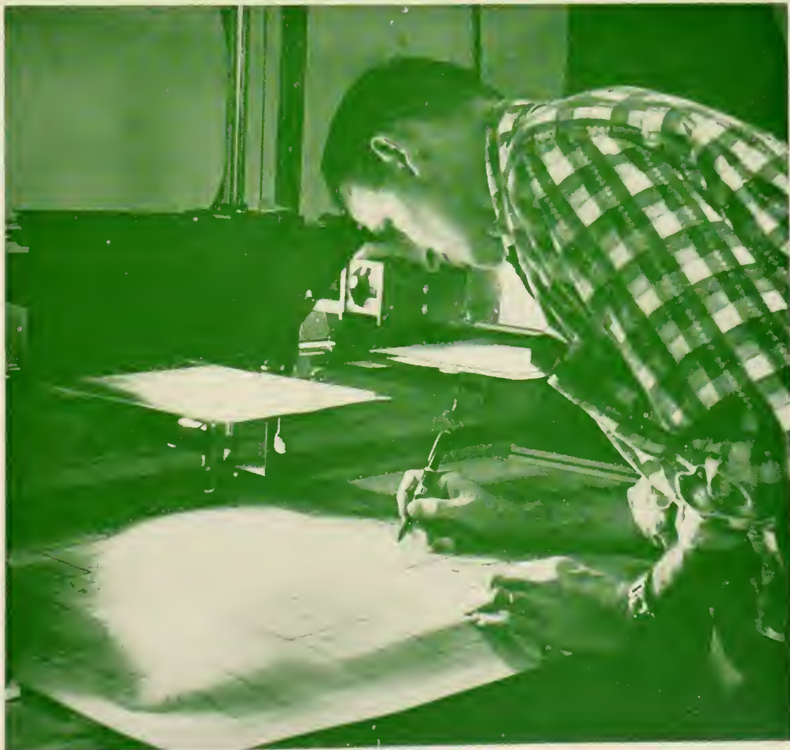
Using a multiscope this forester works on the mapping phase of reclassification on private lands.
